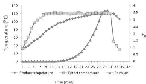
Figure 1. Heat penetration characteristics and  $F_0$  value
